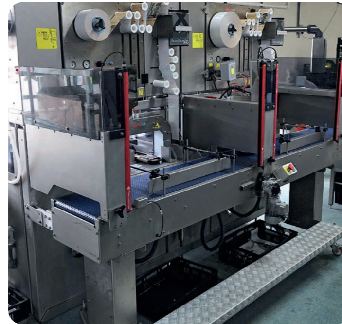
The Bandall TRCS machine at Klooster is a double-headed version that can process a maximum speed 40 packages per minute.
